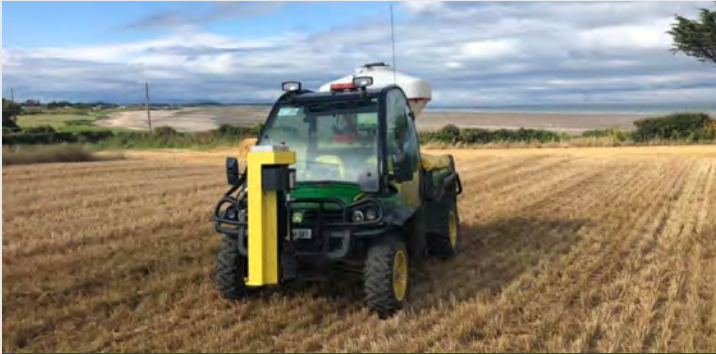
Drummonds soil sampler in action
